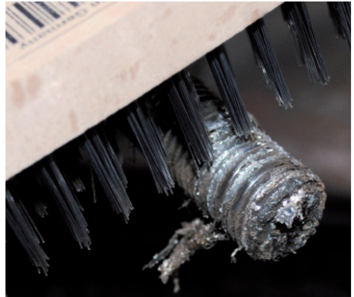
Fig 2. After galvanizing, the fabric tape residue must be removed by means of a wire brush
