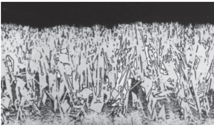
Fig 2. Microstructure of the thick coating obtained using a high silicon steel
